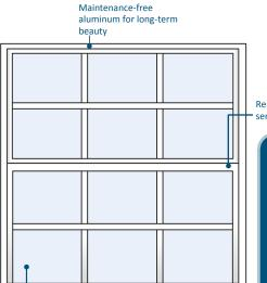
Continuous lift bar on bottom of vent for easy open/close
